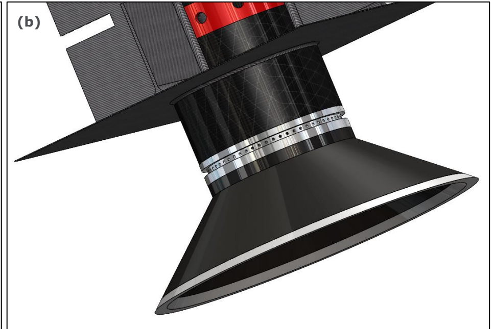
Fig.4 – (a) Primary structure components. (b) Payload Adaptor.
