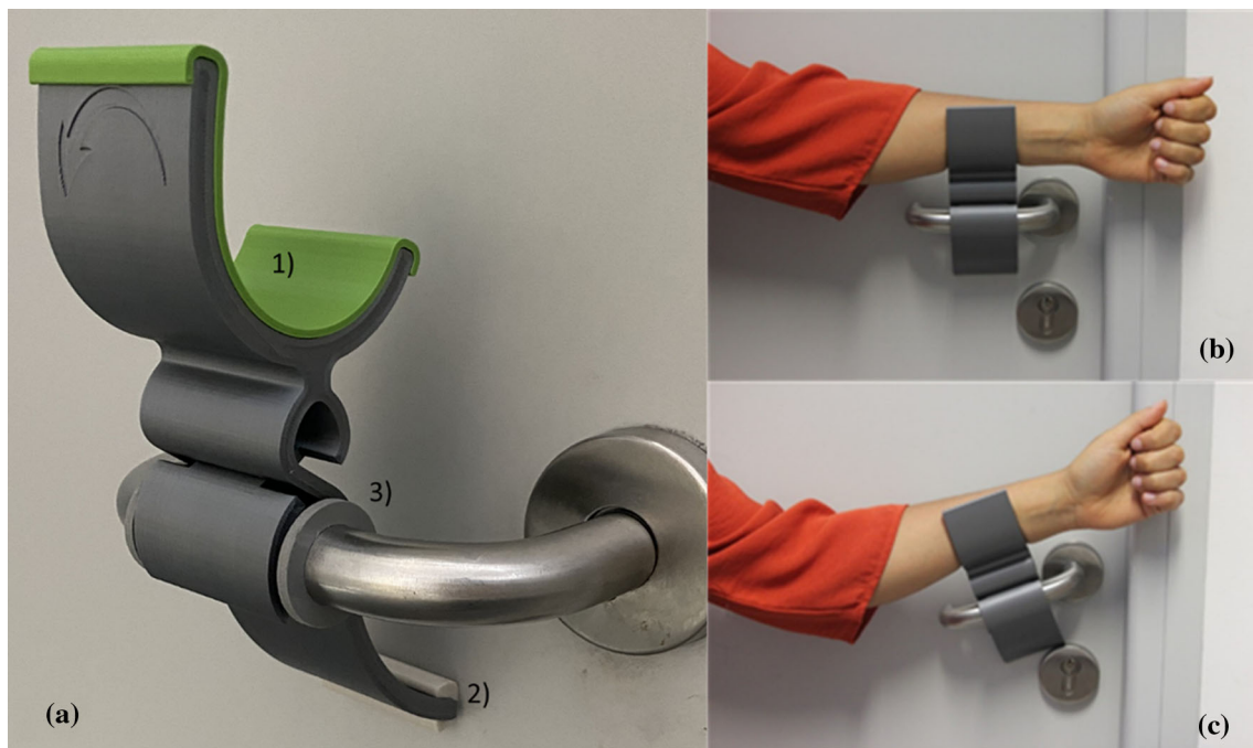
Fig. 6 HANDGENIC improvements: a) Accessory parts of the HANDGENIC to improve functioning: 1) a clean PLA top cover, 2) a soft PLA grip to improve contact with the door; and 3) a TPE grip; b) arm placement c) and the HANDGENIC being used to open a door
