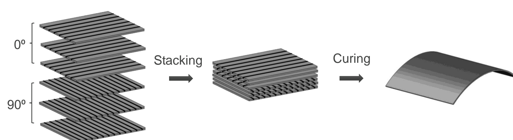
FIGURE 2. Deformation caused by orthotropic coefficient of thermal expansion and chemical shrinkage.
